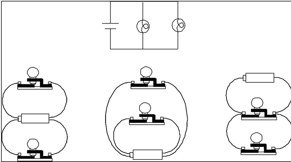
**Figure 1: Three different physical configurations that can be represented by the same circuit diagram.**
