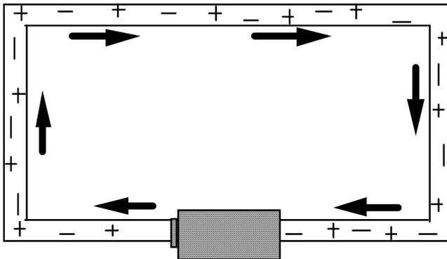
Inserting a battery creates an electrical potential difference
